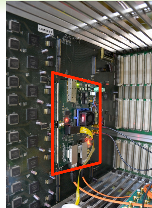
OLC connected to OMB running 12 GBT links at 175
